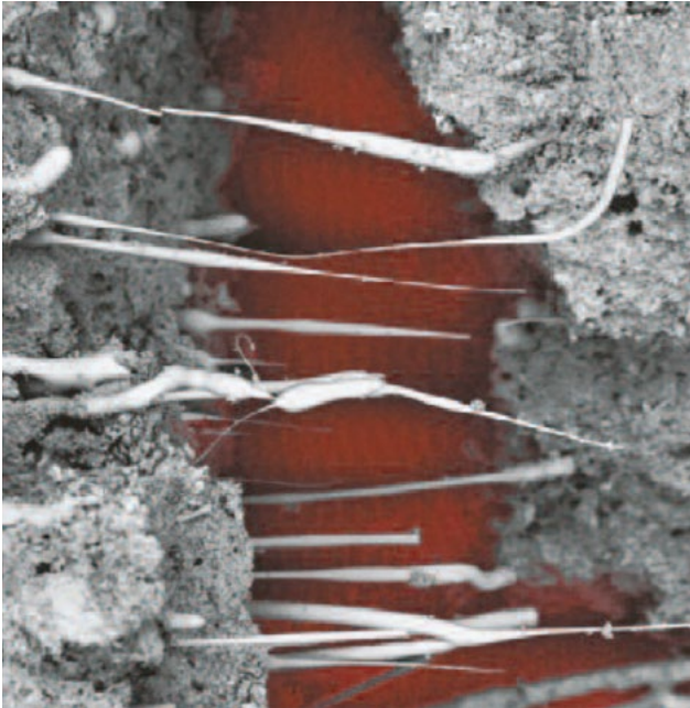
Glass fibres within the core of a Glasroc specialist board
