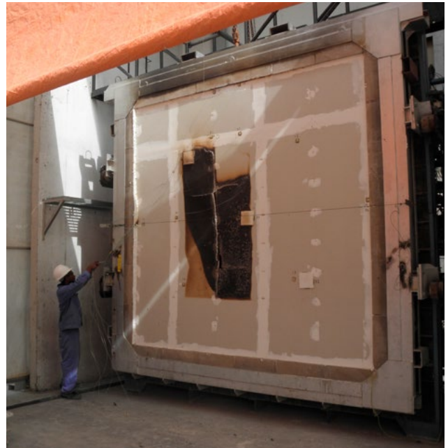
Failure of fire rated partition
