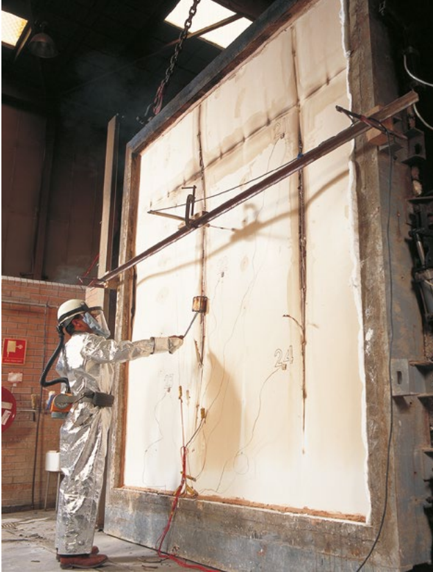
Fire resistance test - integrity testing on 3m high partition
