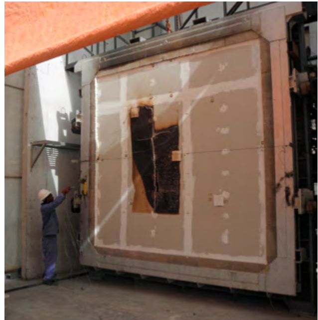
Failure of fire rated partition
