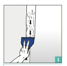
Using a 100mm taping knife, apply a bedding coat of Gyproc\* Jointing Compound to the board joint at approximately 100mm wide and 1-2mm in thickness ensuring that the joint is fully covered.
