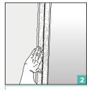
Position Glasroc X\* Tape and embed it into the jointing compound using the taping knife. Remove any excess compound and allow to dry.
