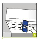
Apply a finishing coat of Gyproc\* Jointing Compound to the corner as smoothly as possible with a 200mm finishing knife, feathering out the final coat 200mm from the nose of the trim. Allow to dry. Sand and paint.
