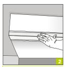
Press Gyproc\* Metal Corner Tape into position and straighten. Firmly embed corner trim using the taping knife or roller. Remove any excess compound and allow to dry.
