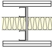
Two Gypframe 'C' Stud frameworks braced at max. 1200mm centres. Studs at 600mm centres. 50mm ISOVER Eco APR in the cavity. Linings as in table.
